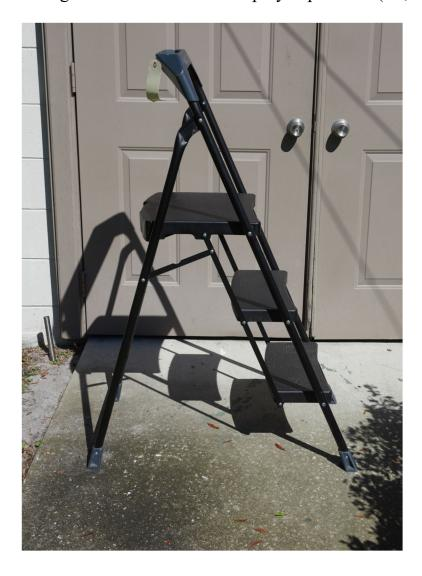
The steps of the step stool have a curved profile on the front edge when viewed from a bird's eye view. (Doc. 34-2 at 3). The front edge of the steps comes closest to the pivot point at the center of each step; the overhang gets larger moving outward from the center, reaching about 1.25 inches from the front edge of the step to the pivot point. (*Id.*).
